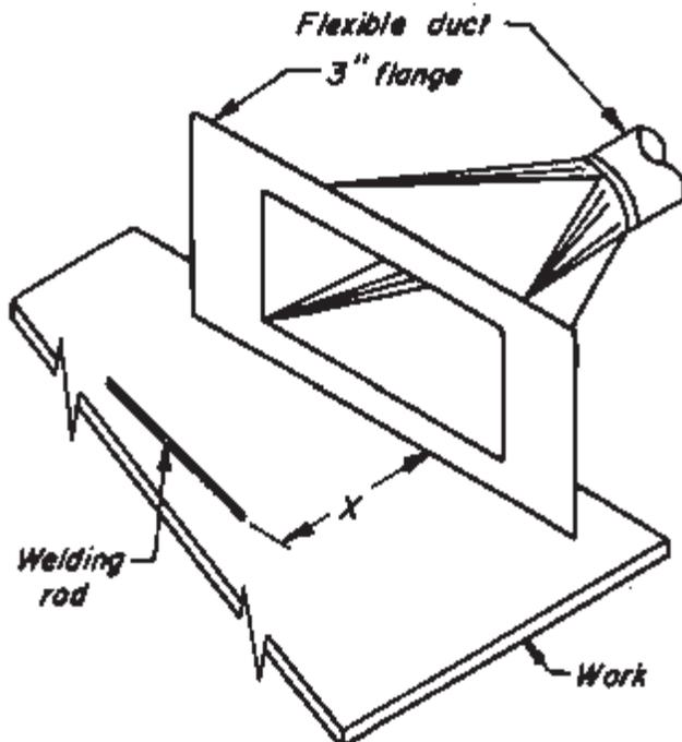
**Figure 18 - Moveable hood for local exhaust**
