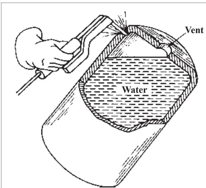
Figure 20 - Safe way to weld a container that held combustibles
